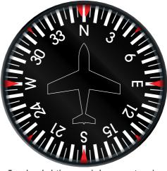
To make calculating crosswind components easier, use the aircraft's Direction Indicator (DI).
