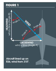
drawing that the crosswind component is the wind speed multiplied by the sine of the angle between the nose of the aircraft and the wind direction (called the relative wind angle). We can also see how the headwind component could be calculated, either as the wind speed multiplied by the cosine of the relative wind angle, or as the wind speed multiplied by the sine of the angle between the beam of the aircraft and the wind direction.
